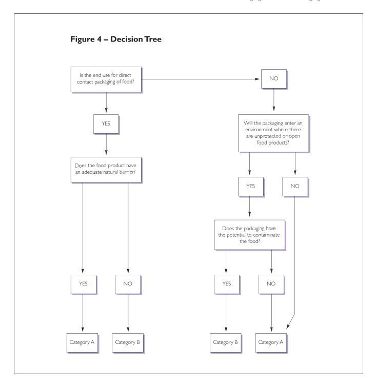
subsequent hazards and to provide an example of their application. Category A provides for a lower-risk category and B for hazards of greater severity.
